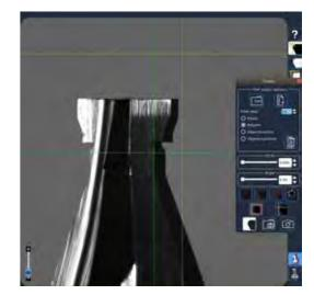
Second front camera (4 camera) allows to have a 90X magnification, ensuring a very small diameter tool visualization. Maximum tool diameter measurable: 120 mm.
